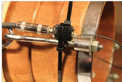
Triggers were mounted using releasable tie-wraps. This allowed for adjustments and movement as needed to find the optimal locations.
