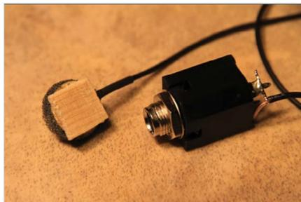
Eight Scheller piezo transducers registered independently record the timing of attacks on each of the eight drums. Each was “sandwiched” between a piece of birch a thin foam pad. They transmitted signals over a ¼” phone jack.
