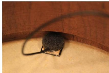
The pickups attached to the underside of each head near the intersection of the head and shell. They were positioned to avoid being directly underneath the striking area (locations shown with arrows above).
