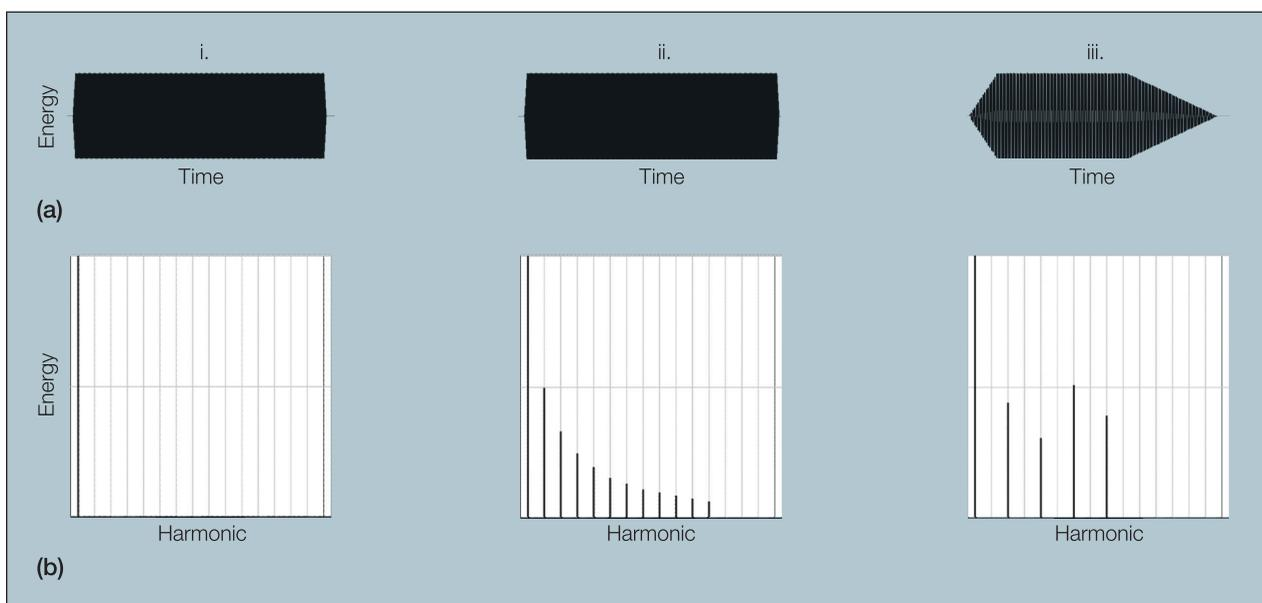
**Fig. 2.** (a) Waveforms and (b) Power spectra: of i. 1000 Hz sinewave; ii. 1000 Hz sawtooth tone, and iii. a single tone with a fundamental of 261 Hz from Power Failure alarm from IEC:2006 [20].
